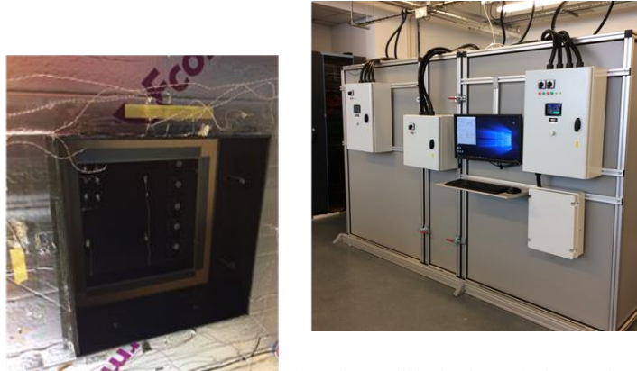
Figure 3: The calibrated hot box with the installed sample
