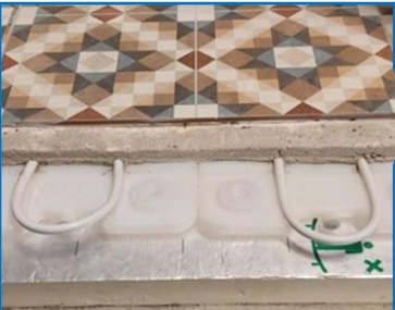
PCM product S21, Melting temperature: 18-36 °C
