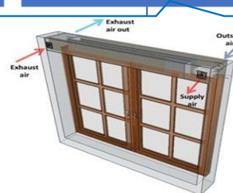
Heat recovery by heat pipe: 76%
