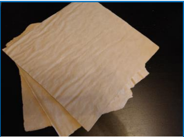
Whole panel thermal conductivity: 0.024 W/mK
