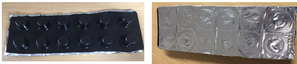
Figure 25 - Blister PCM Panel prototype
