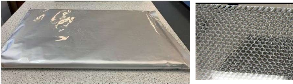
Figure 18 – Aluminium honeycomb panel with INERTEK 23 and Mylar Bag
