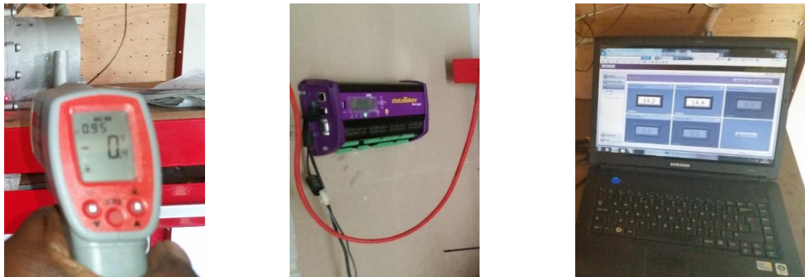
Fig. 20. DT85 data logger , K-thermocouples , Flow meter , Hand help thermometer, and Air flowmeter.
