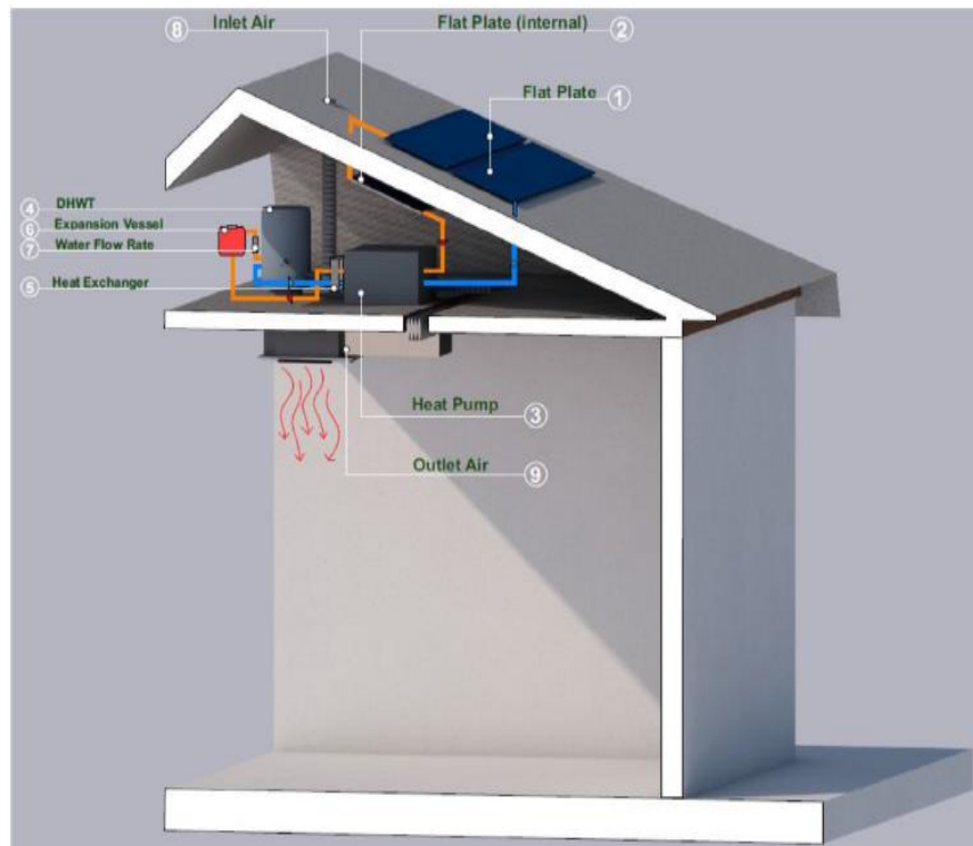
Fig. 8. The system configurations on building's roof
