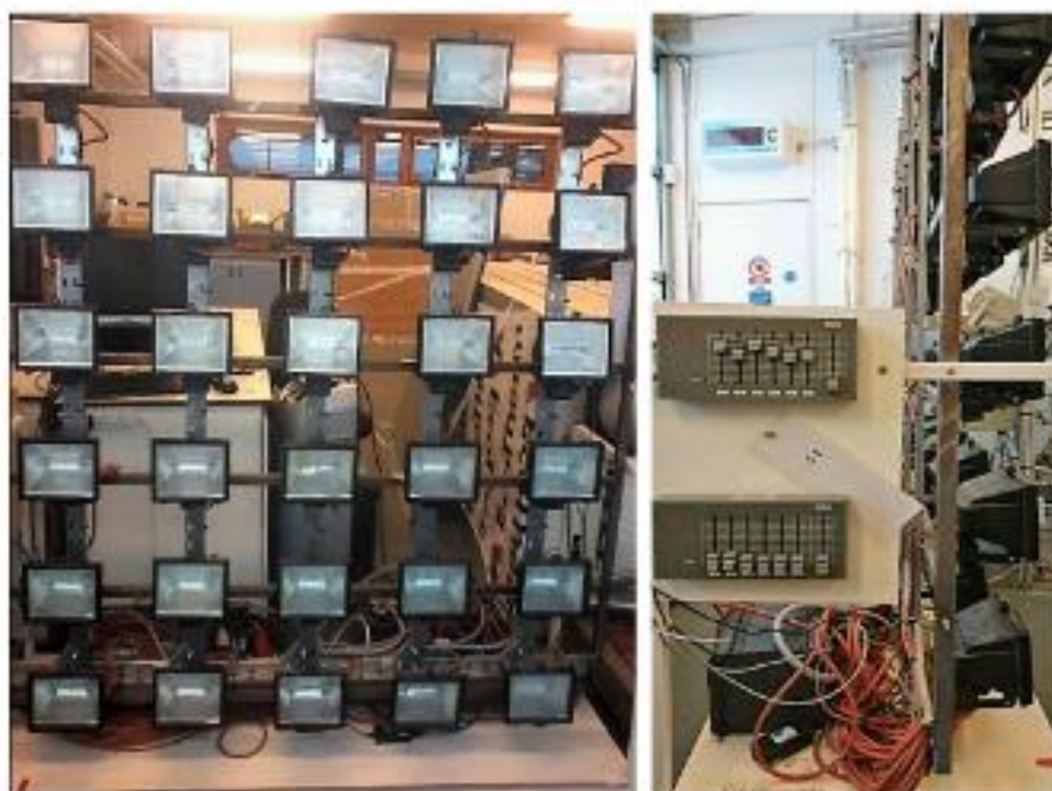
Fig. 11. Solar insolation simulator and light regulator
