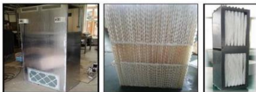
Fig. 1. Cooling units: PEC indirect cooler (left), PEC core (middle) and fibre cooler (right)
