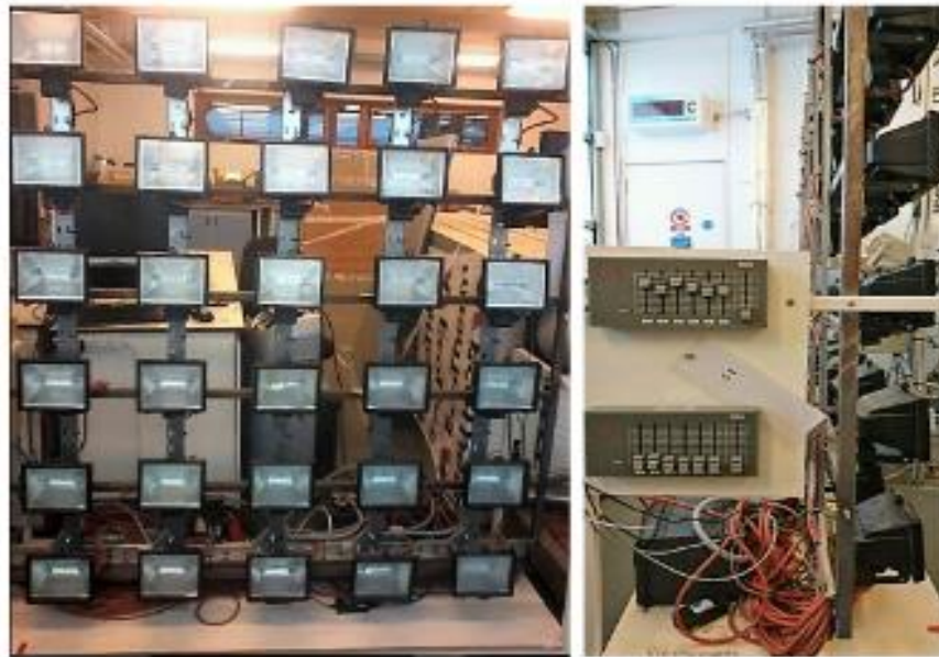
Figure 13 - Solar radiation simulator and light regulator
