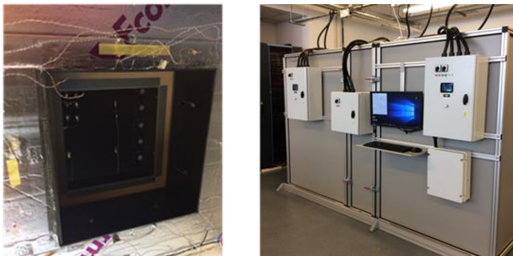
Figure 4 - The calibrated hot box with the installed sample
