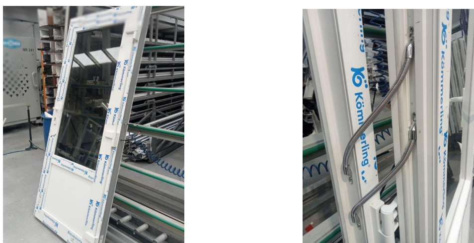
Figure 10 – Photos of the PV Vacuum glazing system integrated in the frames – Spanish demo
