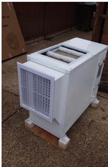
Figure 19 - Installation of the evaporative cooler
